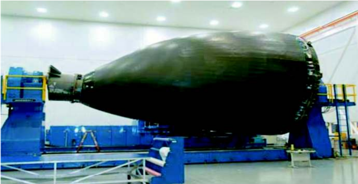
Tooling for large composite aerospace parts, Source: Boeing
