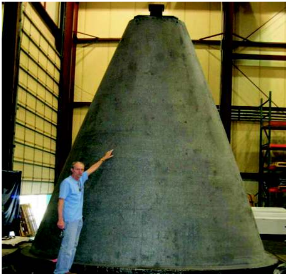
Nova-Tech Engineering (Lynnwood, Wash.), using carbon foam covered with carbon/bismaleimide prepreg. Source: Nova-Tech Engineering
