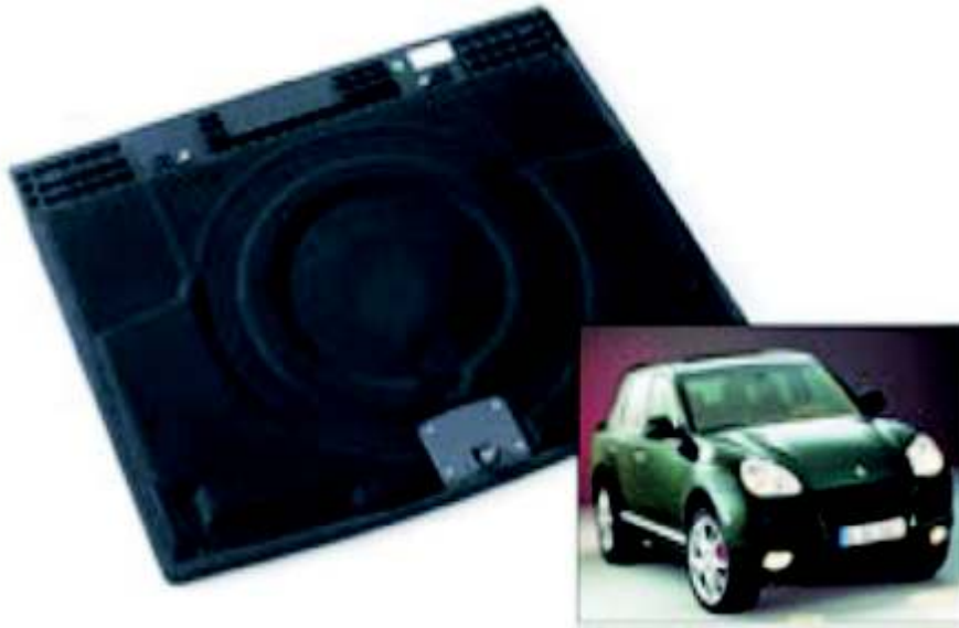
Figure 2: The rear cargo area load floor of the Porsche Cayenne is composed of structural layers of natural fibre composites surrounding an expanded polypropylene foam core and covered with a carpet cloth, Source: Quadrant Natural Fibre Composites
