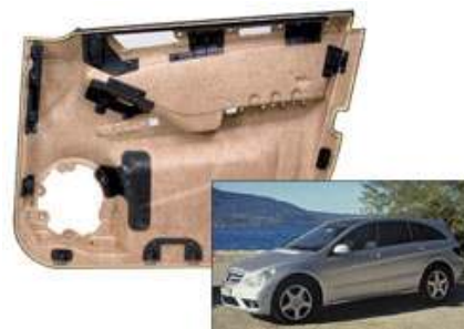
Figure 1: A door panel from the new Mercedes M-Class and R-Class (inset) is made of natural fibres composites, Source: FlexForm Technologies
